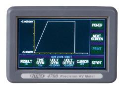
Chart Mode automatically plots voltage readings from a few seconds to several days. Highly useful for determining ramp linearity, overshoot and sag on hipot testers and other HV sources.
