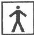
This symbol indicates that the Hydra ECF/ICF device has been classified as a Type BF Applied Part. A BF-Type Applied Part complies with specified requirements of the EN-60601-1 (1988) standard to provide a higher degree of protection against electric shock than that provided by Type B Applied Parts and is marked with the symbol above. Note: Type BF Applied Parts are not suitable for direct cardiac application.
