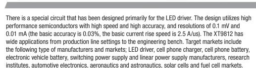
> Six high speed operating modes: 1. Constant Current (CC); 2. Constant Resistance (CR); 3. Constant Voltage (CV); 4. Constant Wattage (CW); 5. Constant Current (CC) + Constant Voltage (CV); and 6. Constant Resistance (CR)+ Constant Wattage (CW)
