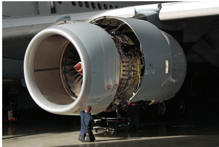
Figure 3. For the technician to understand where to place the balance weights on an engine, the vibration/balancing system must know the engine speed and the phase of vibration
