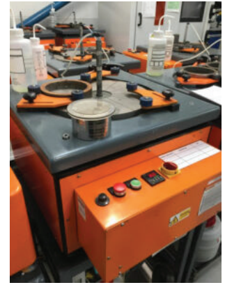
Figure 1. Rotary table for semiconductor wafer lapping.
