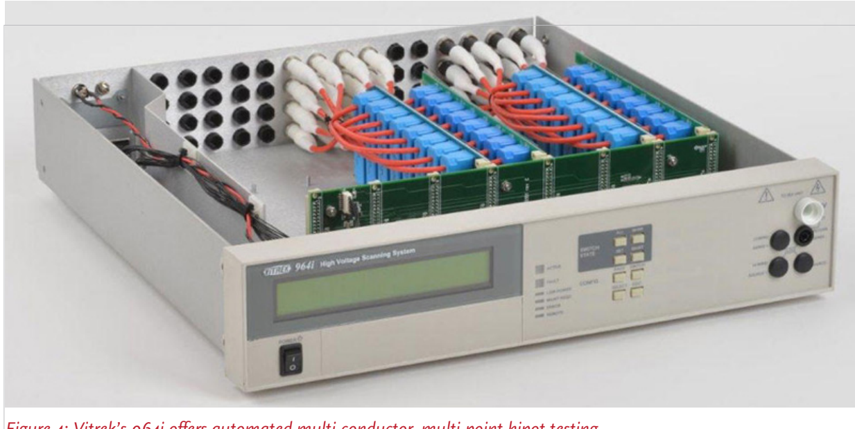
Figure 4: Vitrek's 964i offers automated multi-conductor, multi-point hipot testing.
