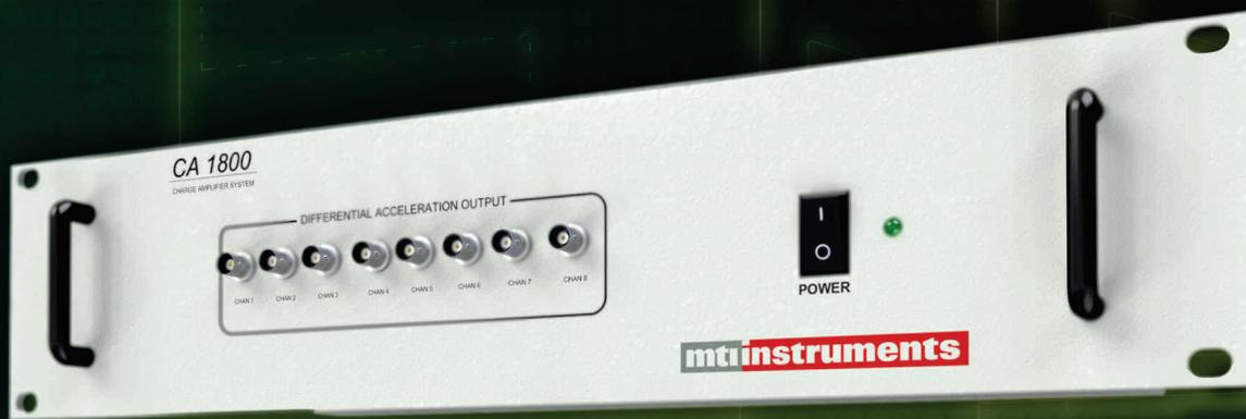
The CA1800 Charge Amplifier System conditions and amplifies charge-mode accelerometer signals. It is a rugged, rack-mountable instrument designed to be used in engine test cell control rooms and other environments where charge-mode accelerometers are used to measure machinery vibration.
