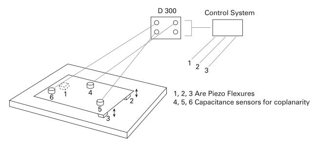
Three gap measuring probes mount to the upper plane (die bonding tool). A control system monitors coplanarity of the tool to the lower plane (die or substrate) and provides position control to the actuators.
