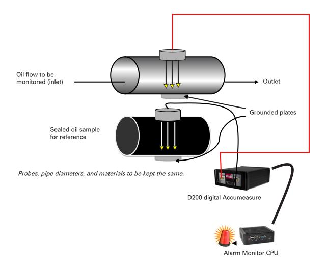
MTI's flexible, off-the-shelf flat probes easily bond to the tube with epoxy to mold to the shape of a plastic/glass oil tube and continuously monitor the capacitance of the oil or oil/water mixture passing through. The company's D200 Digital Accumeasure serves as the monitoring sensor signal conditioner. Immune to thermal drift and easily calibrated to the sensitivity of water in oil, it is available with a digital limit alarm module.
