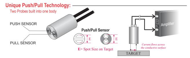
The Push-Pull probe is a unique version of MTl's Accumeasure™ amplifier series. This special design provides accurate surface information for wafer bow and thickness.
