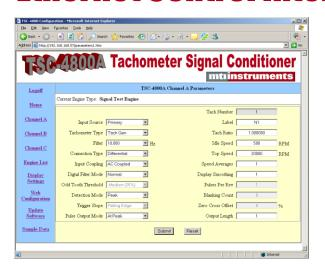
**Web Controls** - The TSC-4800A features a full Ethernet control interface for configuration, control and testing of the unit. A WEB style interface offers users easy access to the unit from any computer running an Internet browser program. Other computers can directly control the TSC-4800A using a simple yet complete machine interface language.
