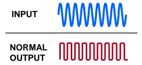
**1/REV OUTPUTS - Pulses coincident with the 1/revolution signal** – Most new engines have an "embedded" 1/revolution signal within the N1 speed signal as illustrated below. The TSC-4800A extracts these "embedded" signals and produces an easy to use 1/revolution pulse which is required for engine balancing.
