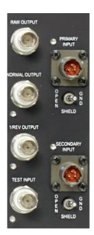
Select between primary and secondary input signals –Many engines have primary and secondary speed signals. Consequently, the TSC-4800A permits the selection of multiple input sources for each channel. Primary and secondary inputs are via three pin MS connectors where a full differential signal can be accepted.
