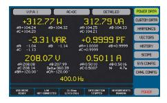
data results (WHr) can also be controlled and viewed from the power data screen. For users with unique data requirements, custom data screens can be built with a spreadsheet application and downloaded to the PA900 via interface or USB drive.
